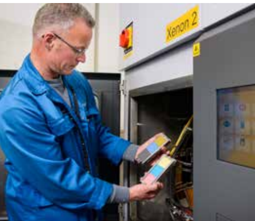
A number of samples are placed in the Xenon weather simulation machine for 3000 hours of extreme testing.
