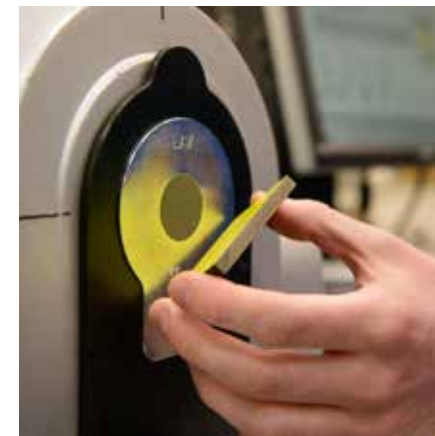
The test sample is scanned three times by a spectrophotometer to make sure the colour reading is accurate.
