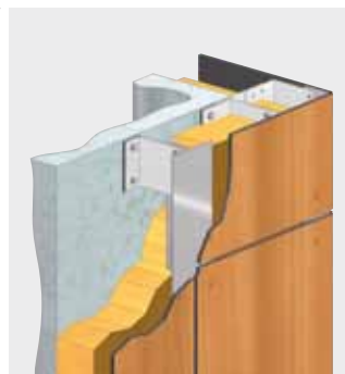
TS700 VISIBLE (EXPOSED) FIXING WITH RIVETS ON A METAL SUB-FRAME
