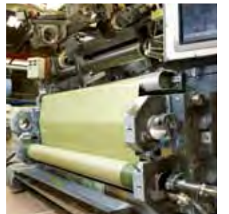
COATING FOLLOWED BY ELECTRON BEAM CURING CREATES AN EXTREMELY SMOOTH AND CLOSED SURFACE
