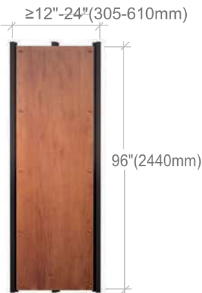
INTERMEDIATE SUPPORT REQUIRED (only 2 rows of fasteners along edge of panel)
