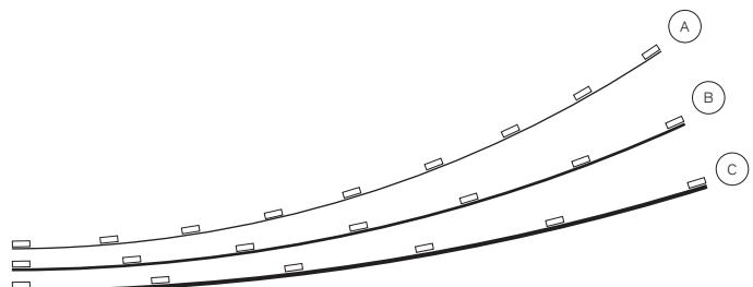
**A.** 6mm thick: radius from 3m to 10m — Espesor 6mm: radio 3m a 10m
