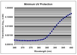
Transmission data obtained using a Shimadzu model UV2401 PC UV/Vis Spectrophotometer.
