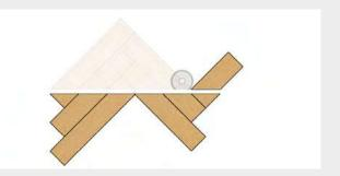
Excess pieces from starting triangles: Dismantle the exess material from the starting triangles. Use it to close the open gaps to the finishing wall. Use the leftover from strips 1, 2 etc. consecutively and cut to size if necessary.
