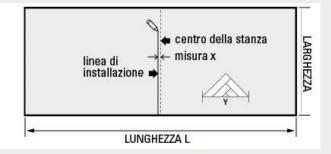
Drawing the installation line. Start from the center of the room. Parallel offset the line using the X measurement as distance.
