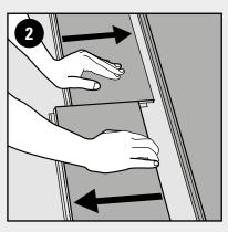
Disassemble the individual slats by sliding them along the short side.
