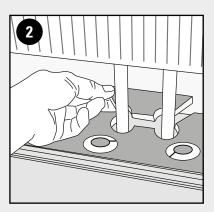
Drill holes at least 15 mm wide in relation to the diameter of the pipes. Remove a small section of stave in order to position the stave. Cover the remaining space behind the pipes with the section removed earlier.
