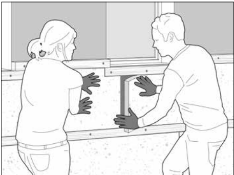
Install insulation in a staggered pattern between the horizontal battens and flush with the timber. Avoid any potential gaps.
