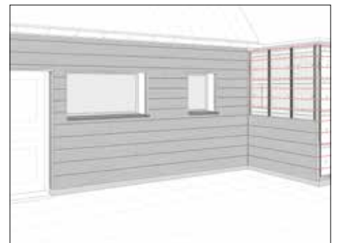
Now finish all other façades, ensuring that the strips meet at the same heights at every corner.
