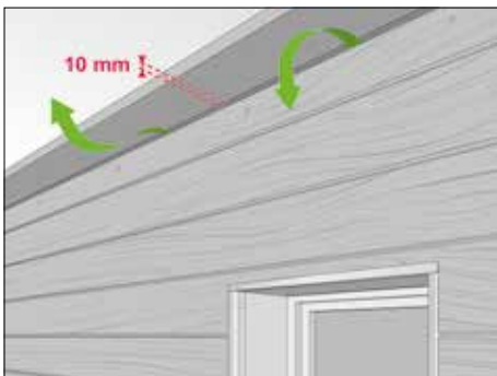
Cut the top of the last strip in the longitudinal direction to the correct height using the saw, being sure to keep a minimally 10 mm gap at the top of the façade.
