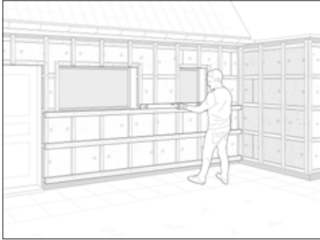
Install another layer of horizontal battens on top of vertical battens.
